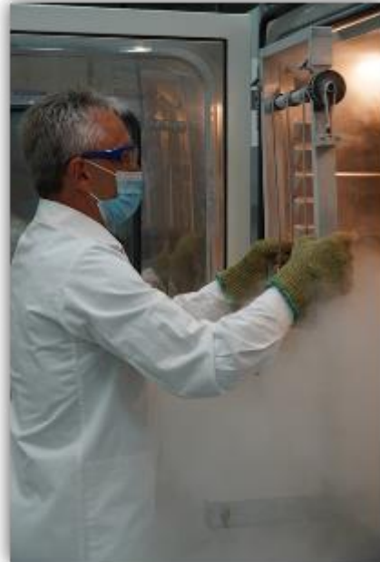
9.17 Cold Bend Test at -80°C 6 mm Mandrel diameter (specified 8 mm)
