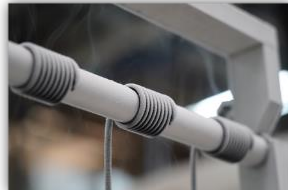
9.17 Cold Bend Test at -80°C 6 mm Mandrel diameter (specified 8 mm)
