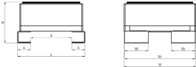
'J' Lead Termination (C-shape)
