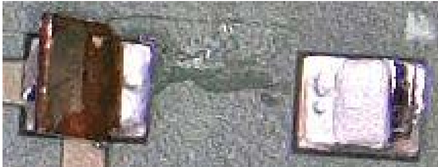
Figure 12: Typical residue pattern after cleaning of tilted SOD
