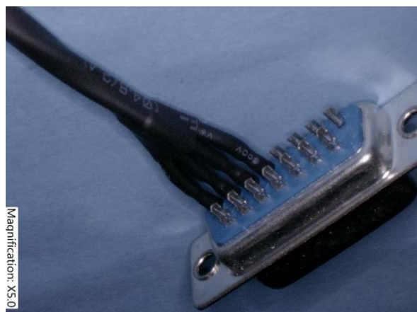
Figure 53: connector and cable after cleaning and shrinking
