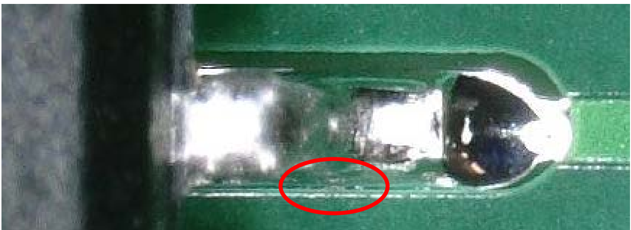
Figure 30: Shifted solder mask pattern with minor residues between lead and edge of solder mask
