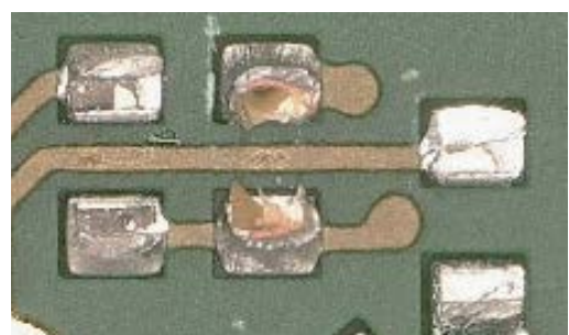
Figure 15: Line under chip – thoroughly cleaning takes 50min. Cleaning the gap under the similar chip w/o line takes y 20min only.
