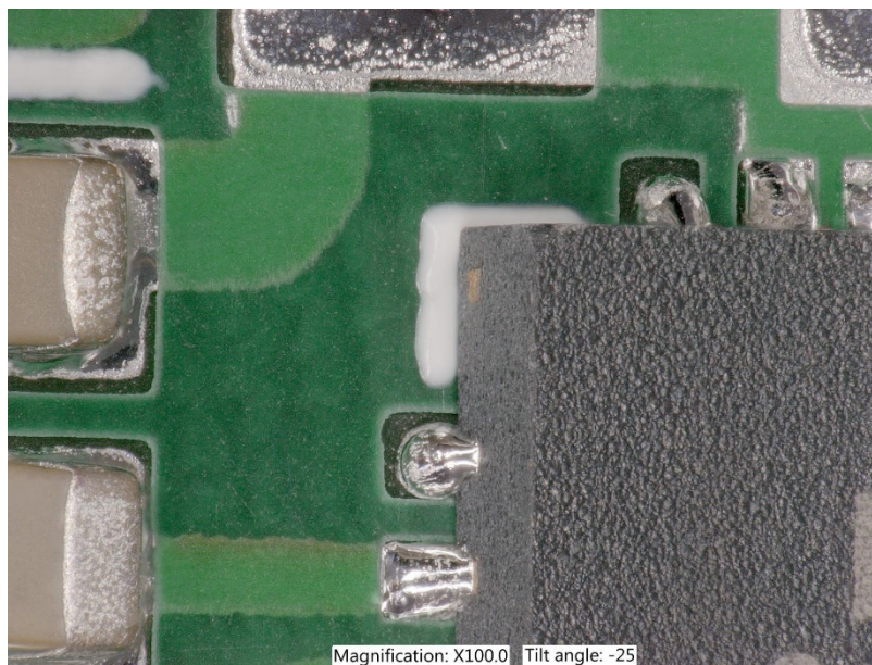
Figure 36: the same QFN after cleaning
