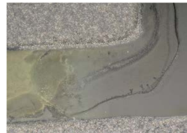
Figure 39: leakage currents on SIR test record and the detailed picture of the same component [2]
