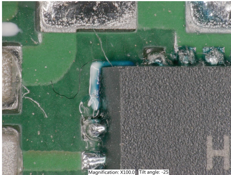
Figure 35: QFN before cleaning
