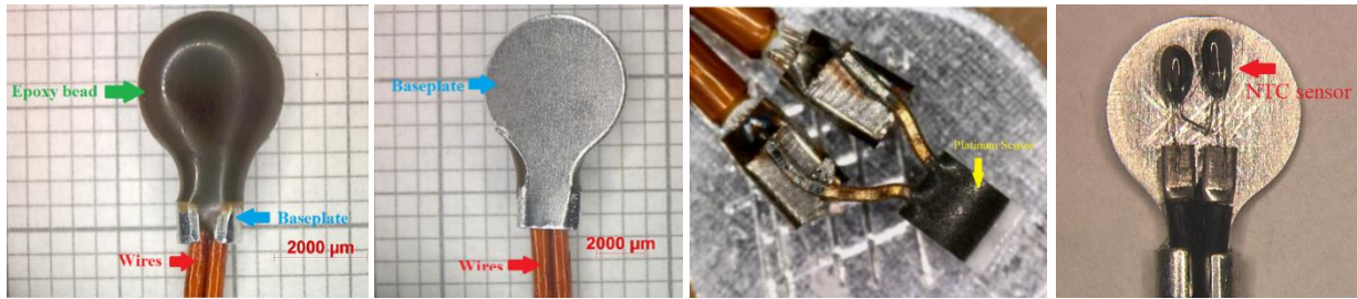
Fig. 1. Details on the construction of the RTD type under study (three first images from the left); internal construction original ESCC-QPL NTC thermistors
