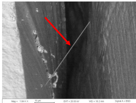
Fig. 6: Whisker link two metal surfaces
