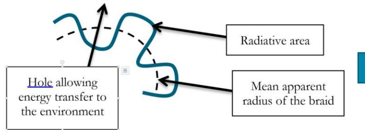
**Geometrical representation of the shielding braid**
