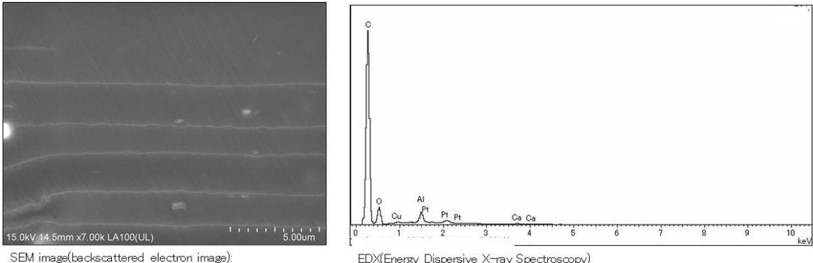
EDX point (b): internal electrode, metallized film
