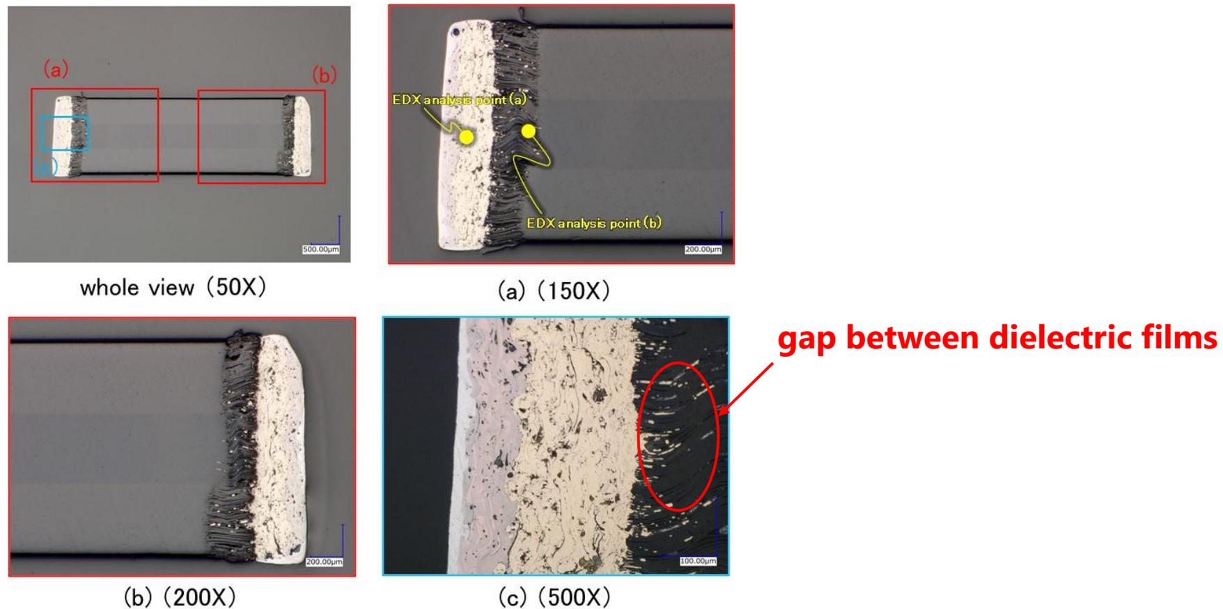
Fig. 12. The result of cross-section observation of stacked metallized film chip capacitor
