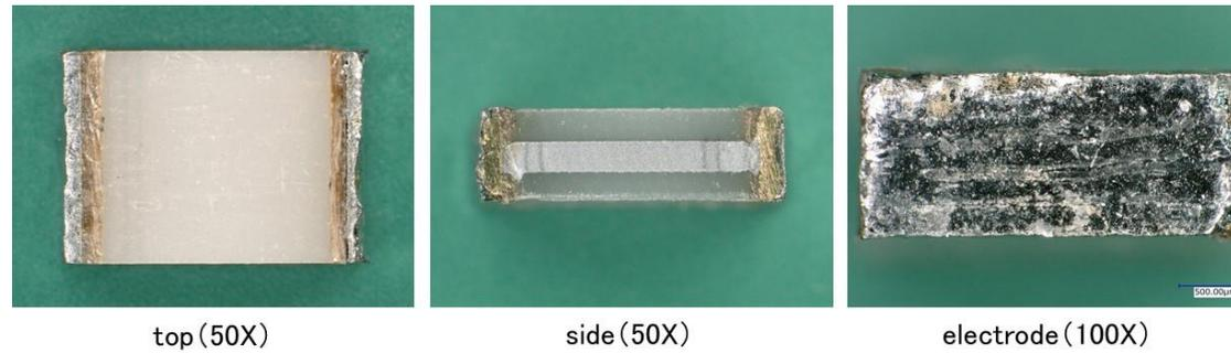
Fig. 10. The result of external visual examination of stacked metallized film chip capacitor
