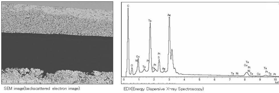
EDX point (a): electrode, conductive adhesive, tantalum element
