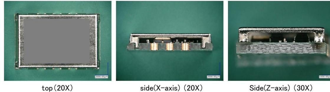
Fig. 14. The result of external visual examination of voltage-controlled crystal oscillator
