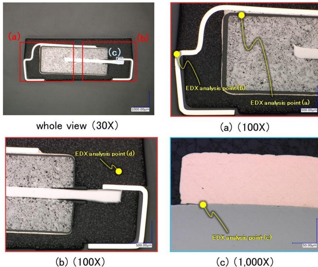
Fig. 4. The result of cross-section observation of polymer tantalum capacitor
