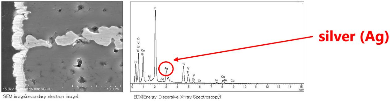
EDX point (c): external and internal electrode, ceramic body
