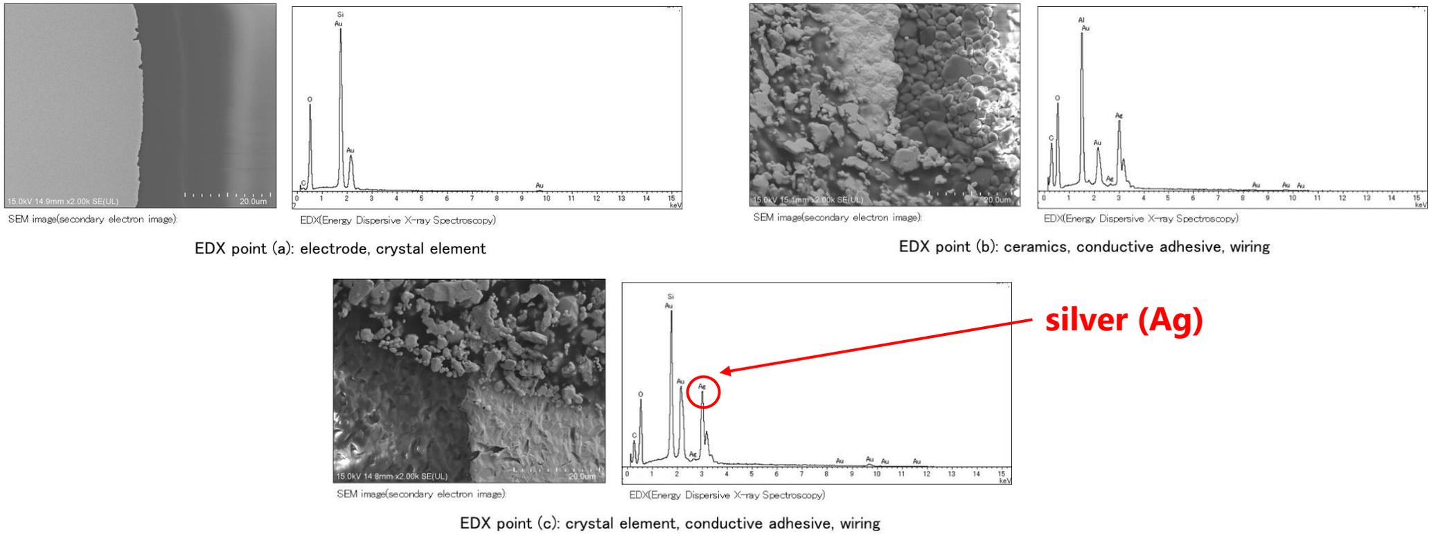
Fig. 17. The result of SEM / EDX analysis of voltage-controlled crystal oscillator
