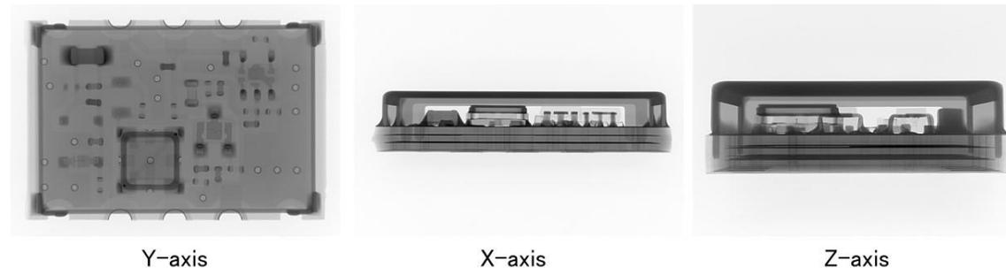
Fig. 15. The result of radiographic examination of voltage-controlled crystal oscillator
