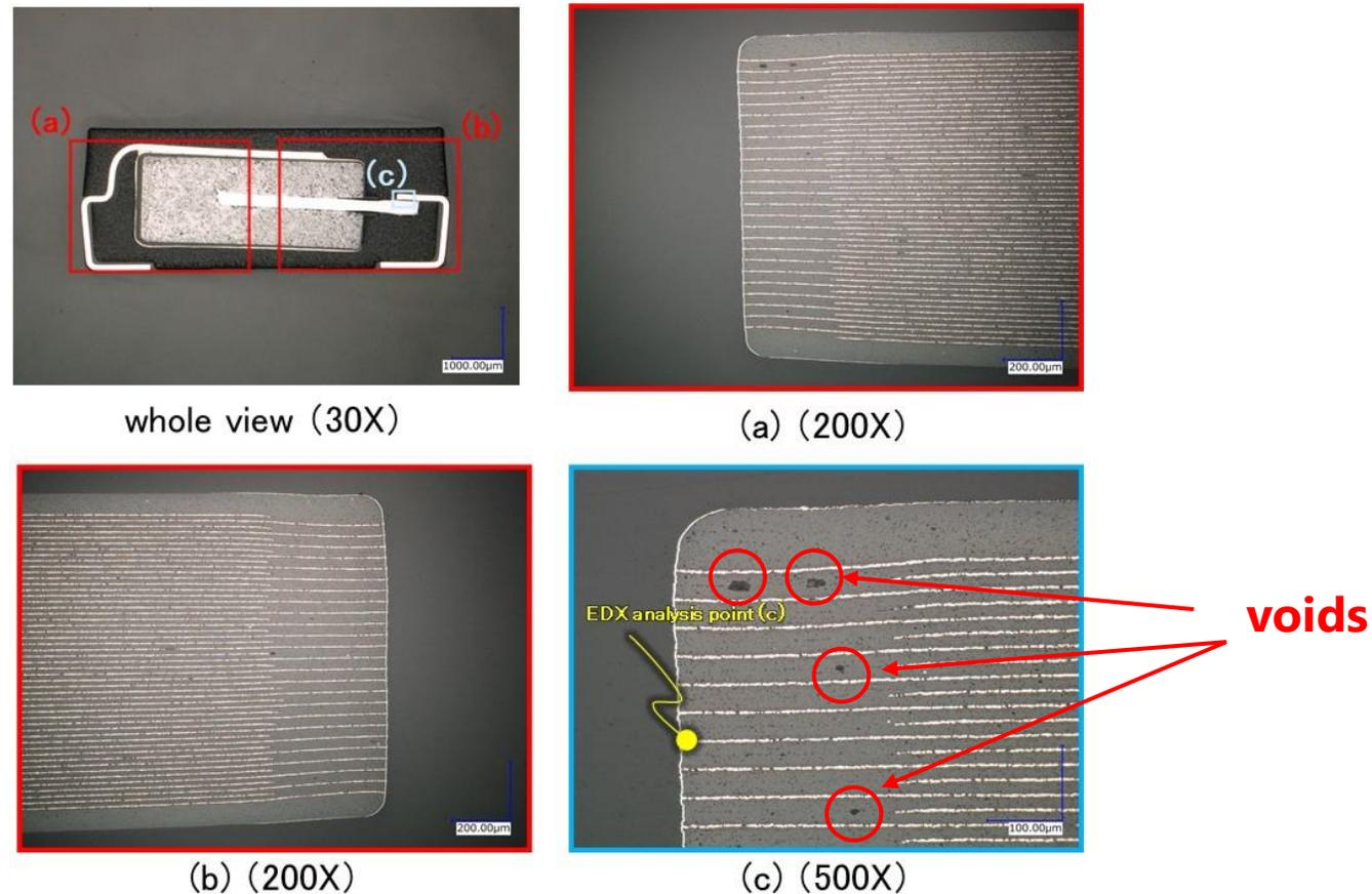
Fig. 8. The result of cross-section observation of solid state battery
