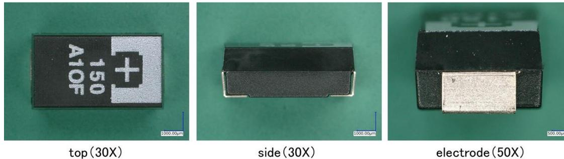
Fig. 2. The result of external visual examination of polymer tantalum capacitor
