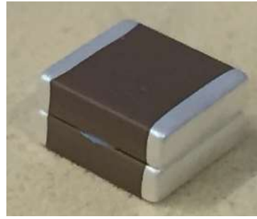
Fig. 10: 2 chips 2220 size stacked with line barrier
