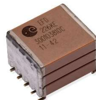
Fig. 2: Stack leaded part (high cap for this example)
