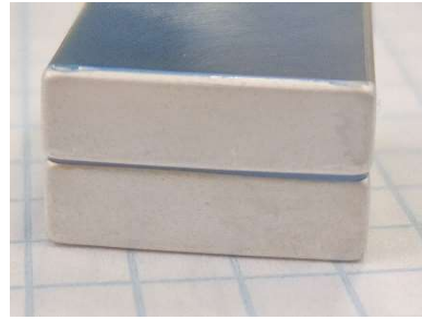
Fig. 7: Glass full-filled preliminary tests after sintering
