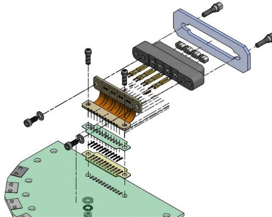
Fig. 12. Representation of flat **MicroMach** connector assembled with Axon's interposer solution
