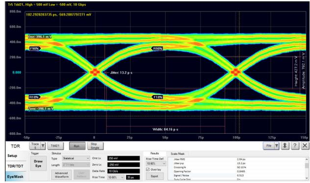
Fig. 10. Eye Pattern for 10Gbps data rate over 75cm of cable over **MicroMach-Flat**<sup>®</sup>
