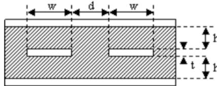
Fig. 5. Representation of a differential stripline structure
