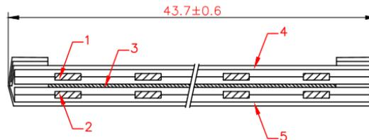
Fig. 3. Definition of a shielded AWG22 FFC pair
