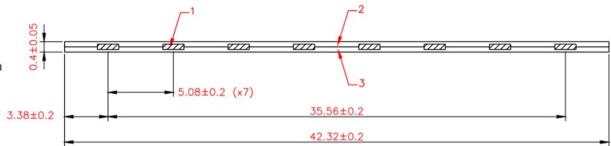
Fig. 2. Definition of AWG22 FFC cable
