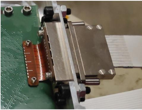
Fig. 9. PCB flat **MicroMach**<sup>®</sup> Connector connected with flat **MicroMach**<sup>®</sup> harness
