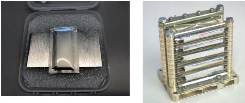
Figure 4: a VACNT pouch on the left (manufactured by NawaTechnologies) and on the right ALMATECH Bank of Supercapacitors.
