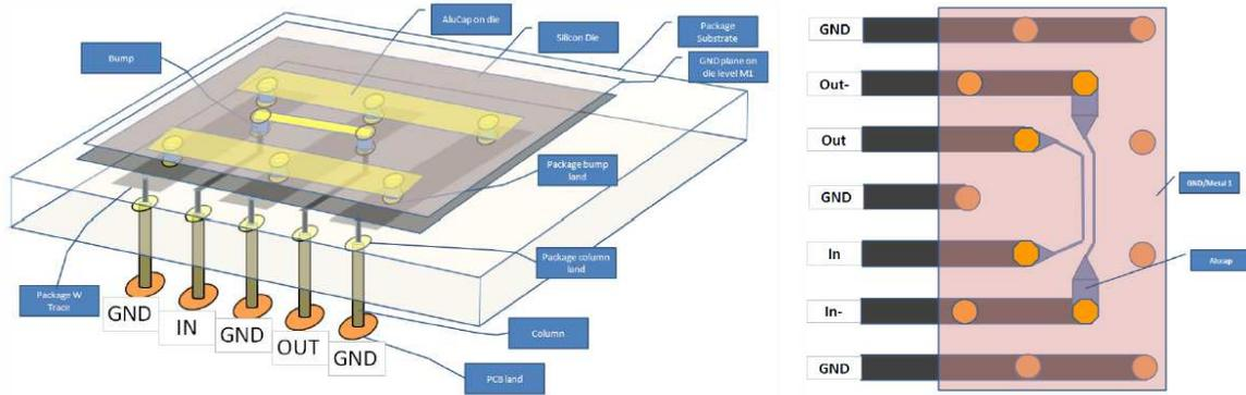
Fig. 5 : HF1 (left) and HF2 (right) routing overview
