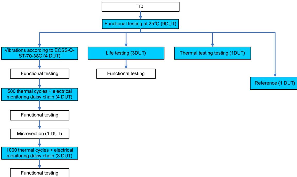
Fig. 4. Synoptic of the test campaigns
