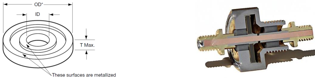
Fig. 3. Discoidal Capacitor Metallization (left), Bulkhead Filter Cross Section (right)
