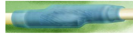
Double Sleeving over soldered connection
