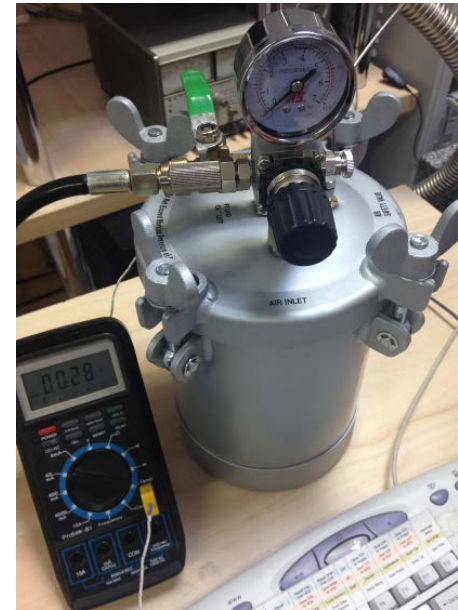
In-house temperature controlled pressure chamber
