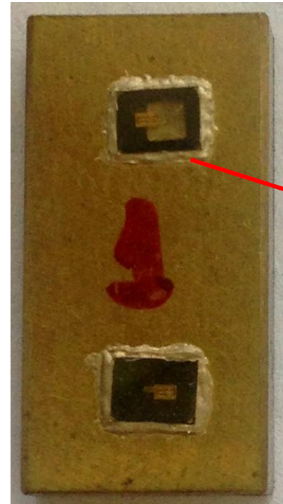
Structures mounted on a carrier to be placed in the pressure chamber (c)
