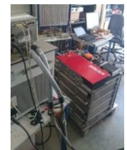
Hybrid Truck pack during testing
